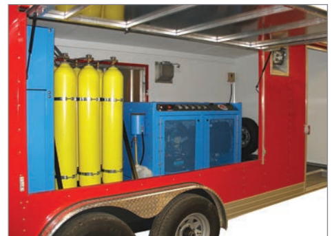
Fully Enclosed Breathing Air Trailer with Fill Compressor, Air Storage Cylinders, and Fill Containment Station
